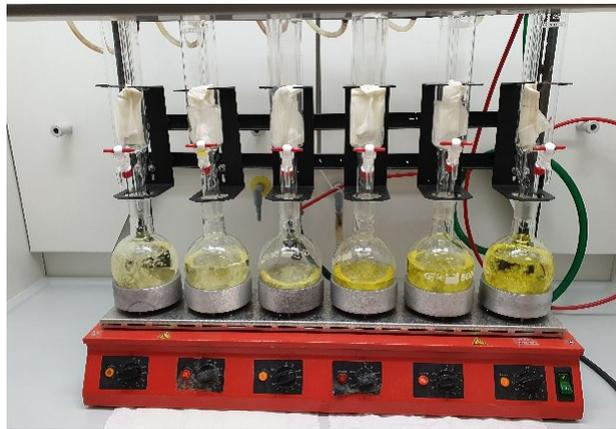
**Figura 8:** Extractor de Soxhlet.
