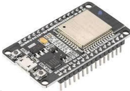
Fig.2.3. ESP32 fonte: [https://www.espressif.com/en/products/socs/esp32\(2024\)](https://www.espressif.com/en/products/socs/esp32(2024))
